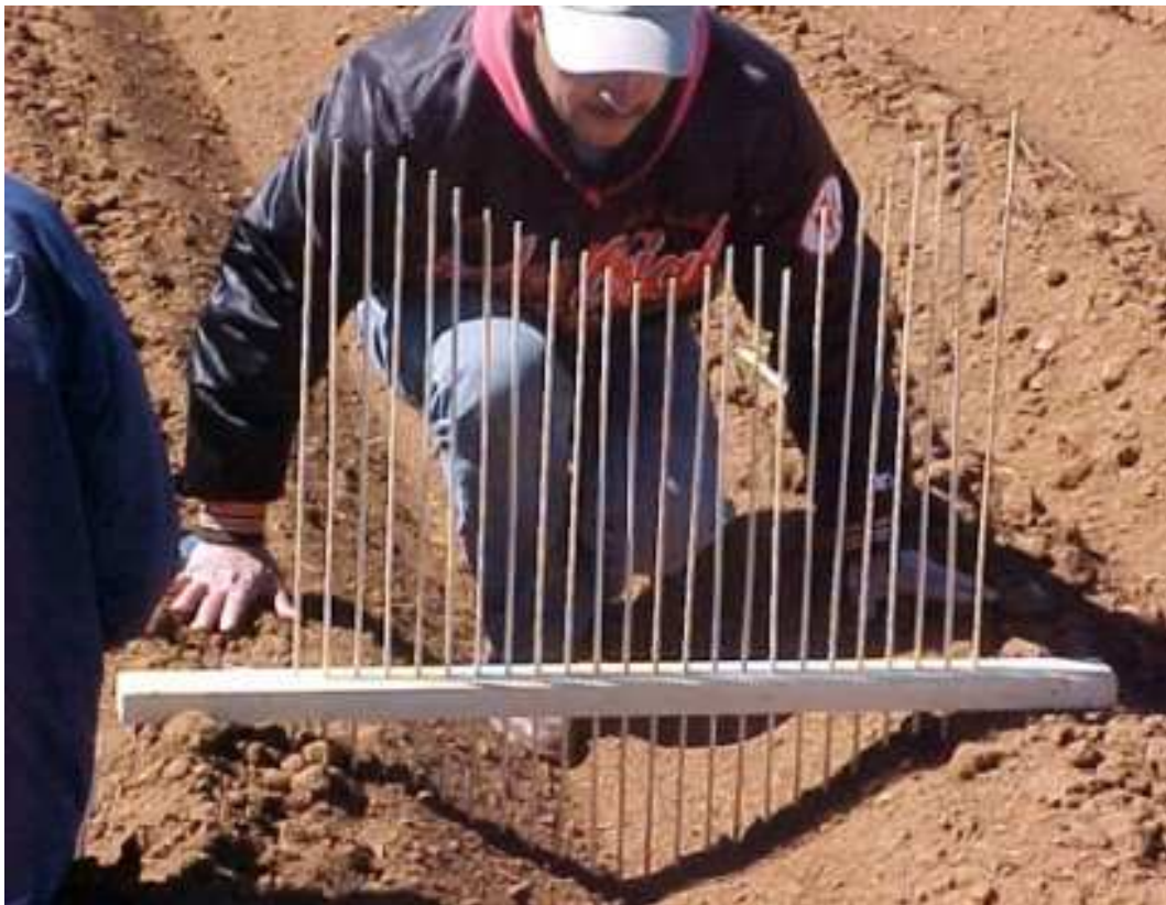
Picture 1. Furrow profilometer for determining cross-sectional area
