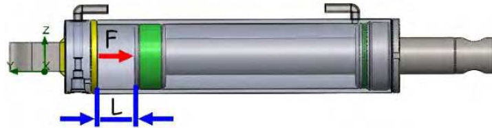
Fig. 7. Operating volume of the hydraulic cylinder
