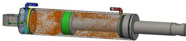
Fig. 15. General view of the flow trajectories inside the hydraulic cylinder
