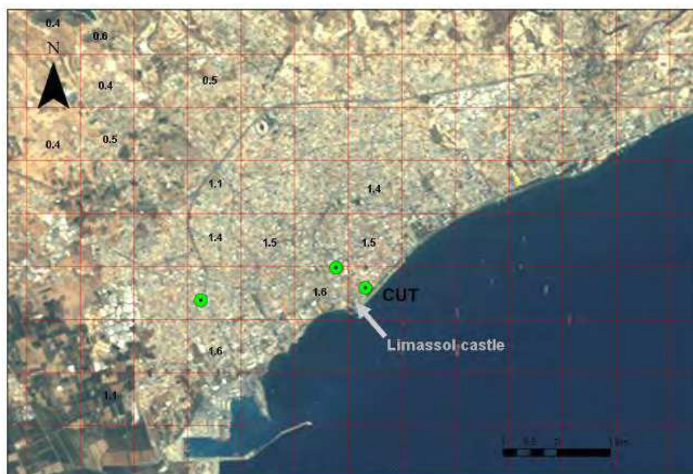
Fig. 16. AOT map from Landsat TM images using indirect method such as the application of atmospheric correction (Themistocleous et al., 2010).
