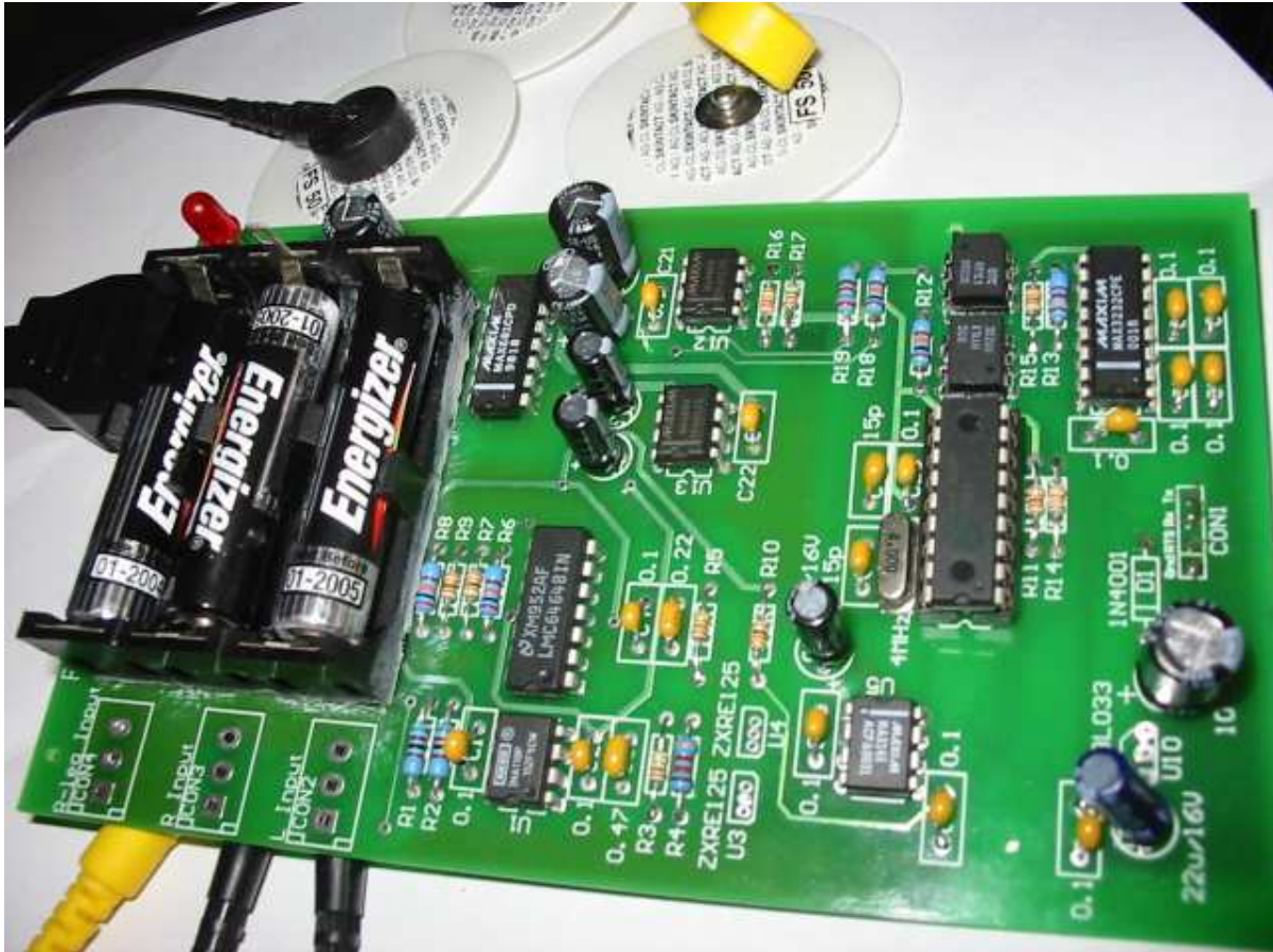
Fig. 20. The actual PC-based Electrocardiogram (ECG) recorder as - Internet appliance
