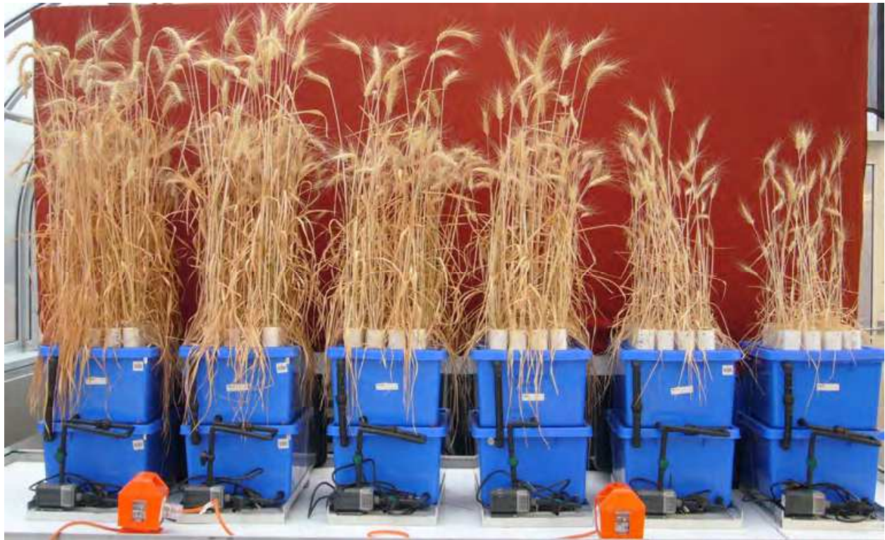
Fig. 7. Flood-drain supported hydroponics in 20 L containers and tubes, showing the appearance of bread wheat plants grown at different concentrations of NaCl to maturity (from left to right: 0, 50, 75, 100, 150 and 200 mM NaCl).
