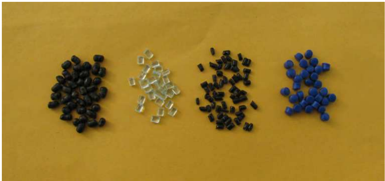
Fig. 2. A selection of plastic fragments suitable for use as a supporting substrate in flood-drain hydroponics.
