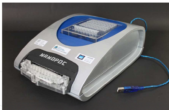
Fig. 12. Point of care electrochemical immunosensing platform Nanopoc®, designed for the diagnosis of foot-and-mouth disease, brucellosis, and Chagas disease (Longinotti et al., 2011). The sample preparation is carried out in the blue sector, which involves magnetic separations. The final amperometric measurement is carried out in the 8-channel electrochemical cells at the front of the device. Data are processed by a PC via a USB connection.
