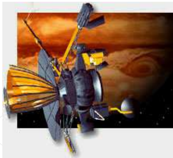
Fig. 16. Galileo's Undeployed HGA.
