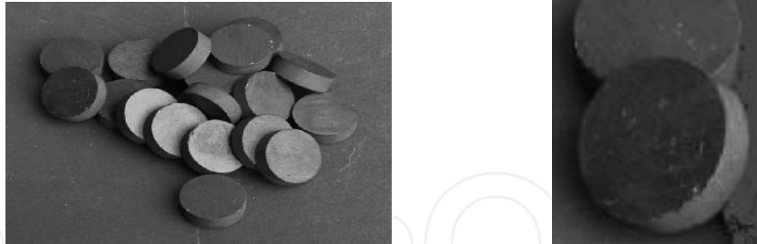
Fig. 4. Disc shaped CIM Mn-Zn ferrite samples (diameter d=16\text{mm} , thickness t=5\text{mm} ).
