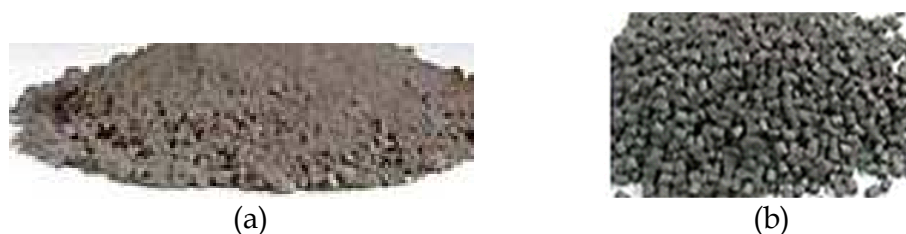
Fig. 3. Mn-Zn ferrite: powder (a) and feedstock (b).
