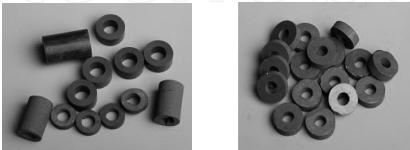
Fig. 5. Ring shaped CIM Mn-Zn ferrite samples (outer diameter d_o=15\text{mm} , inner diameter d_i=6\text{mm} , thickness t=5\text{mm} ).
