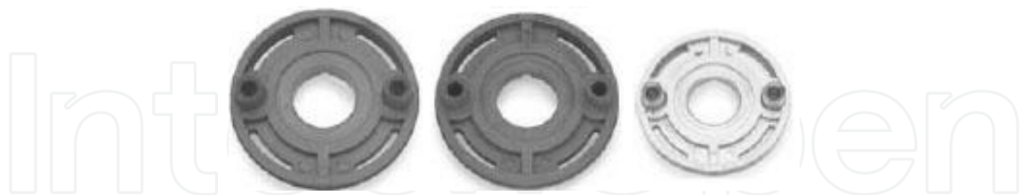
Fig. 2. CIM component: green body, brown body and sintered part, respectively.
