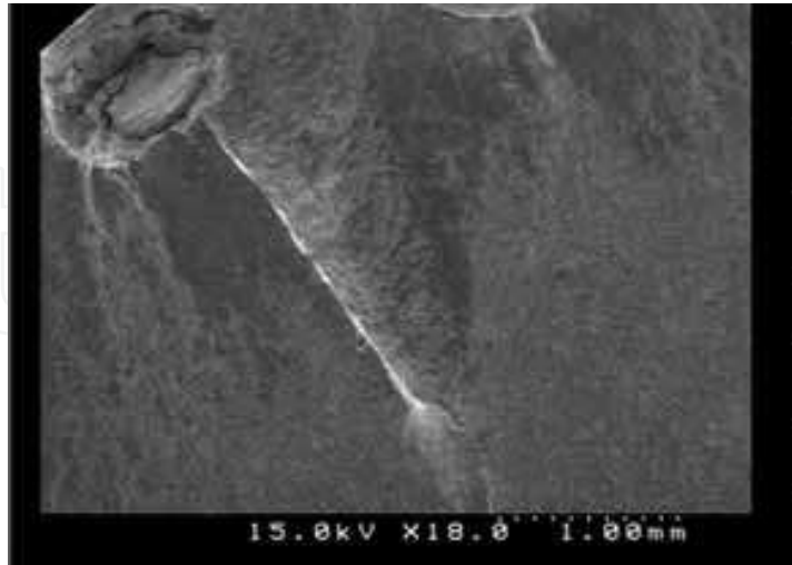
Fig. 43. Fatigue propagation area
