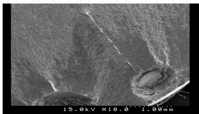
Fig. 4. Fatigue failure arrester at interior pitting deep
