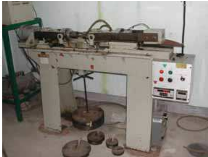
Fig. 39. Rotating bending fatigue test machine
