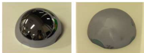
Fig. 4. Photos of the hemisphere specimen: (a) before etching and (b) after etching (etching temperature = 61 °C).
