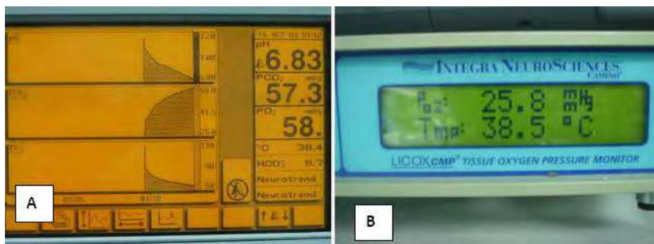
Fig. 11. A: Neurotrend and B: Licox system. Neurotrend is capable of measuring brain temperature, brain pH, P_{tiO_2} , P_{tiCO_2} and HCO_3^- whereas Licox only measures P_{tiO_2} and brain temperature.
