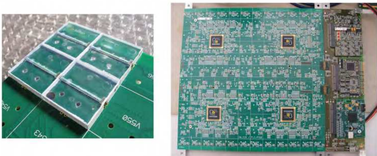
Fig. 14. (left) Four scintillation tiles assembled on the bottom of the HBU. The top side of the HBU. (right) has the front-end electronics with 4 ASICs and calibration LEDs for 144 tiles. The HBU is connected from right to DIF (bottom), CALIB (middle) and POWER (top) boards.
