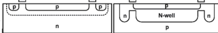
Fig. 5. Double low-doped n-well structure with gates (left) and guard rings and control gate signal (right). Termination techniques (4) and (5) in table 3, respectively.
