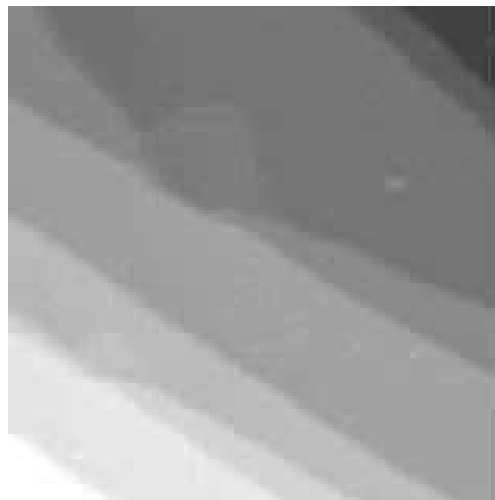
Fig. 14. 200 x 200 nm 2 STM image of the Pt(111) surface taken before any contact has been made between the tip and sample. A series of single atom steps, 0.22 \pm 0.01 nm in height, are observed. Two of the steps are seen to be pinned by contamination, which is likely carbon that has diffused to the surface region from the bulk during processing of the crystal. The image was acquired for an I-V converter gain of 10^8 under the following tunneling condition: tunneling bias of 0.1 V (sample negative) and a tunneling current of 160 pA.
