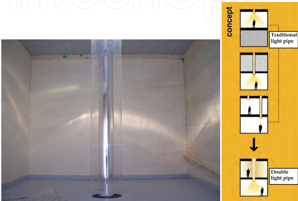
Fig. 1. Reduced scale prototype of a DLP and the concept of the system
