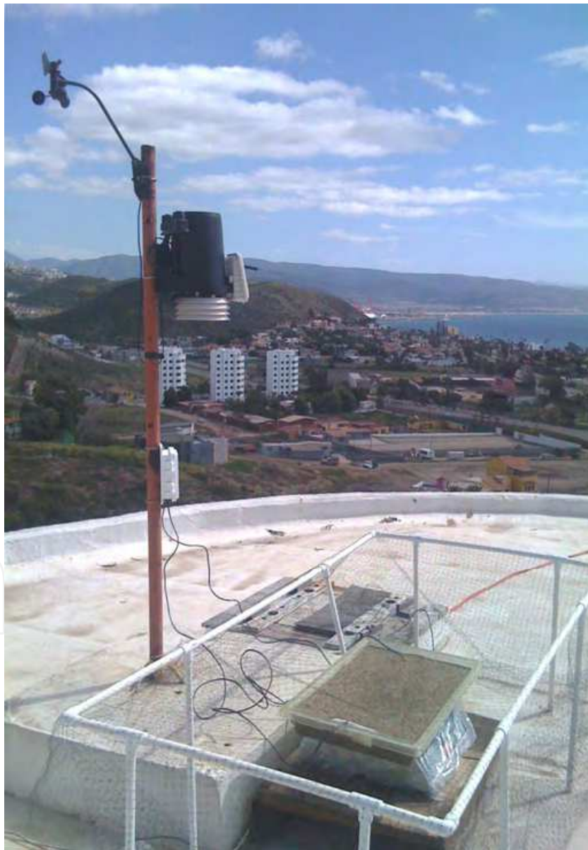
Fig. 1. The experimental setup: the meteorological station, the evaporative tray and the weighing scale used in the study.
