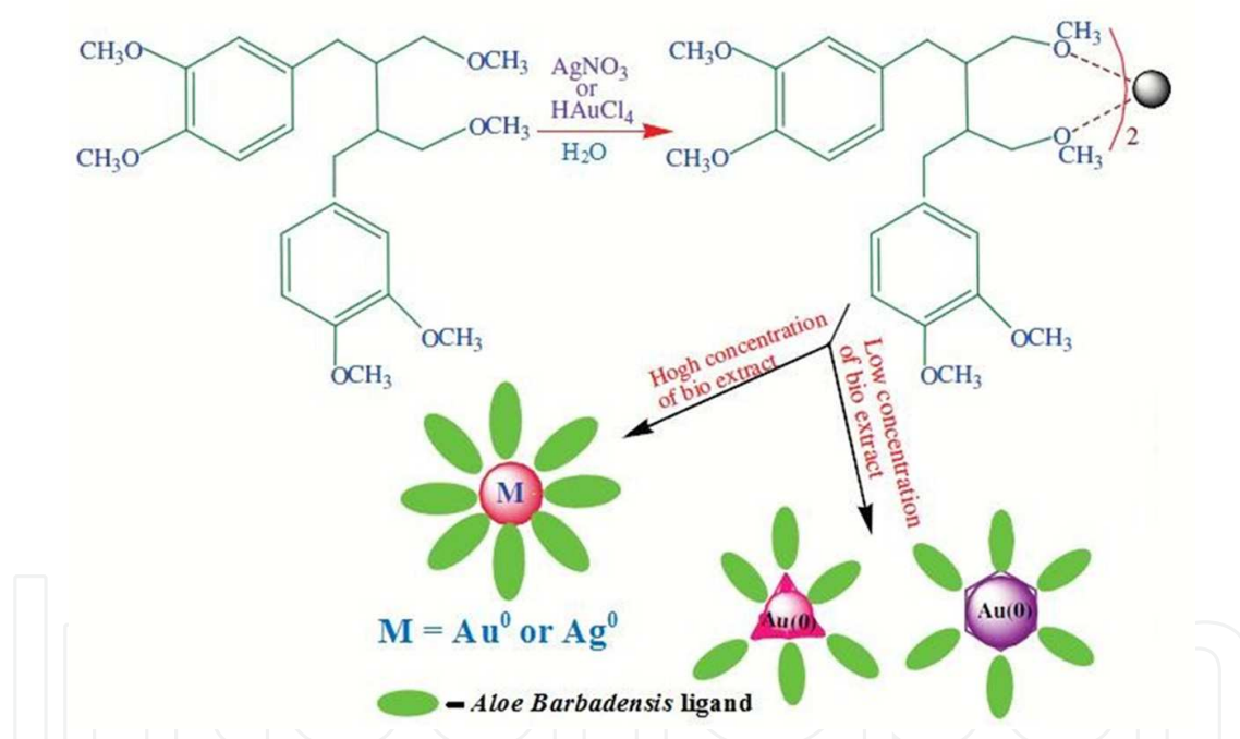
Scheme 2. The presence of small amount of Aloe Barbadensis leads to slow reduction of \text{HAuCl}_4 ions which facilitated the formation of triangular- or hexagonal-shaped nps. Whereas greater amount of Aloe Barbadensis leads to higher population of spherical nps and was confirmed from TEM analysis.
