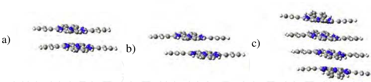
Fig. 2. DFT calculated optimized structures of H 2 Pc dimers and tetramer. In the figure, a) \alpha -modification of H 2 Pc dimer b) \beta -modification of H 2 Pc dimer c) \alpha -modification of H 2 Pc tetramer, respectively.
