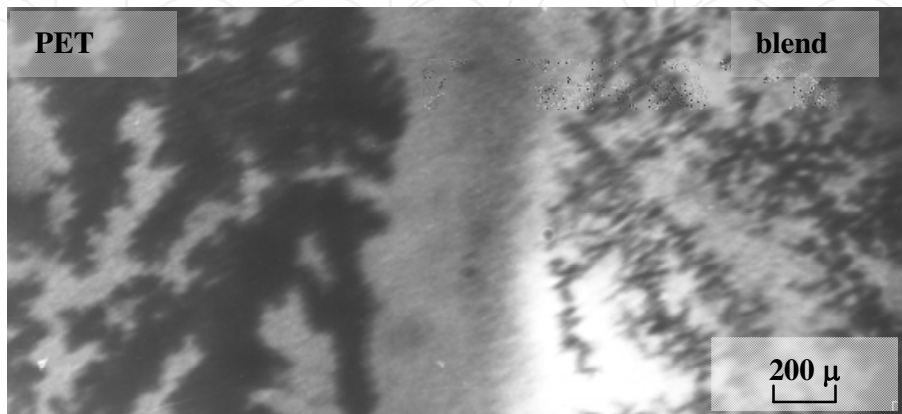
Fig. 19. Micrograph of the diffusion zone at contact of PET with mechanical blend PET/5% of PEN.
