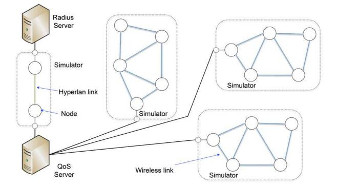
Fig. 16. A schema for the simulation of QoS server impact.
