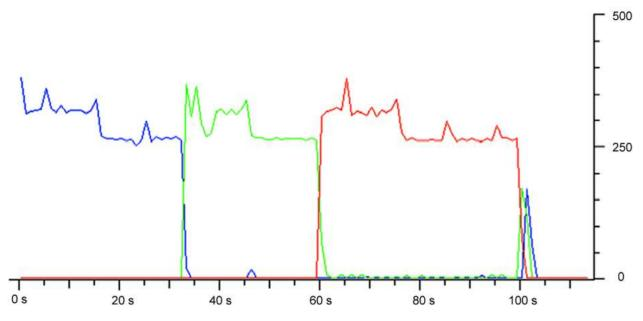
Fig. 9. TCP concurrent flows with QoS (bit/s).
