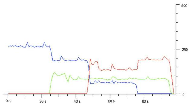
Fig. 10. TCP concurrent flows with bounded bandwidth QoS (bit/s).
