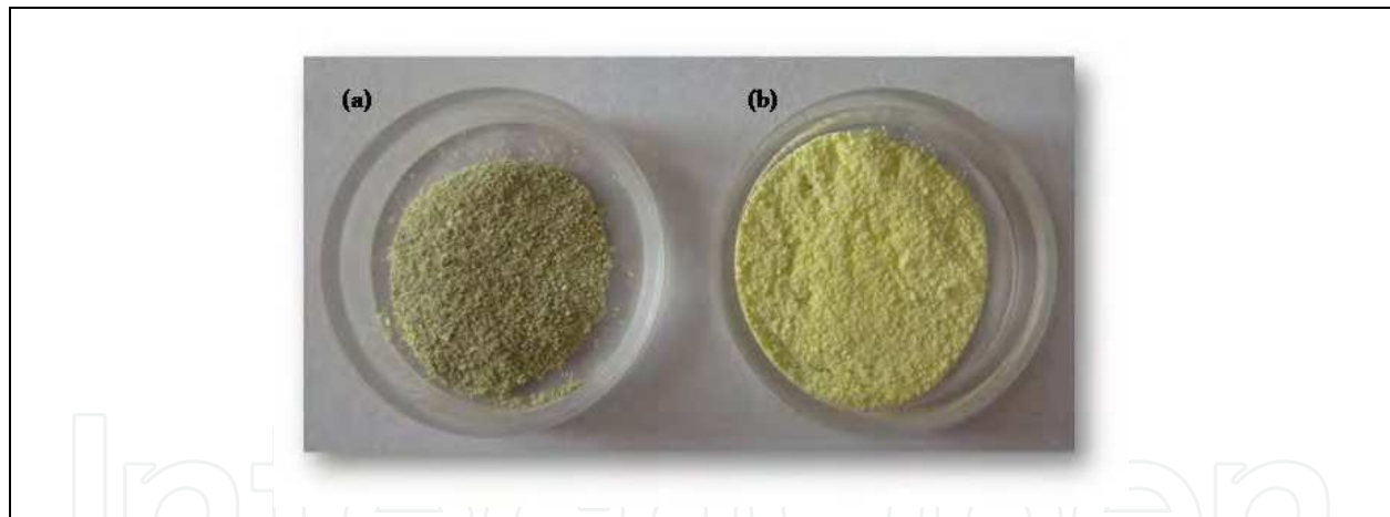
Fig. 3. Picture of as-synthesized YAG:Ce powder before(a) and after(b) post-calcination at 1000°C for 2 hours.
