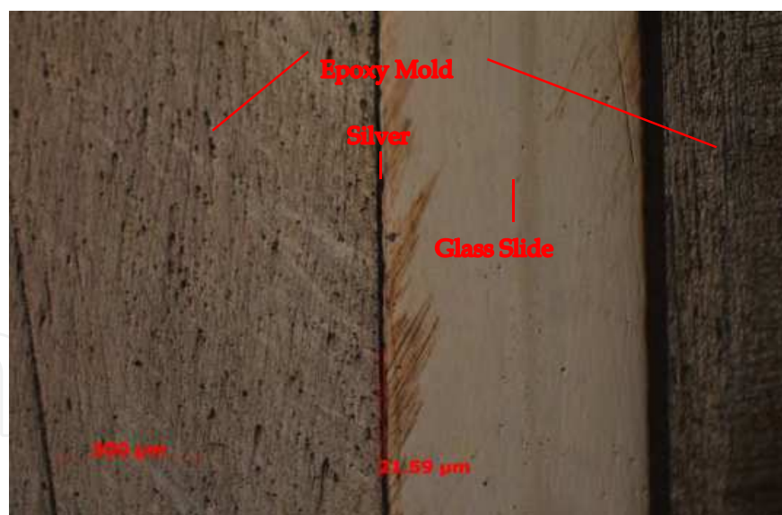
Fig. 3. Optical cross section of the V2 silver on a glass slide in an epoxy mold.
