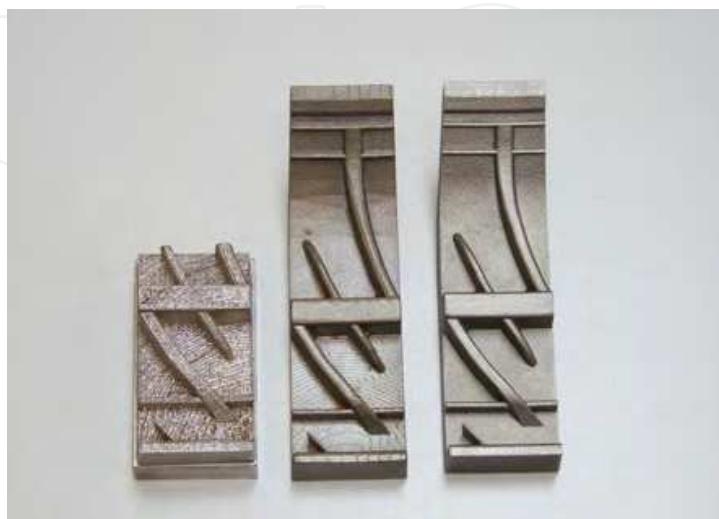
Fig. 6. The one-pitch-segments made by SLM, SLS and DMLS technology.
