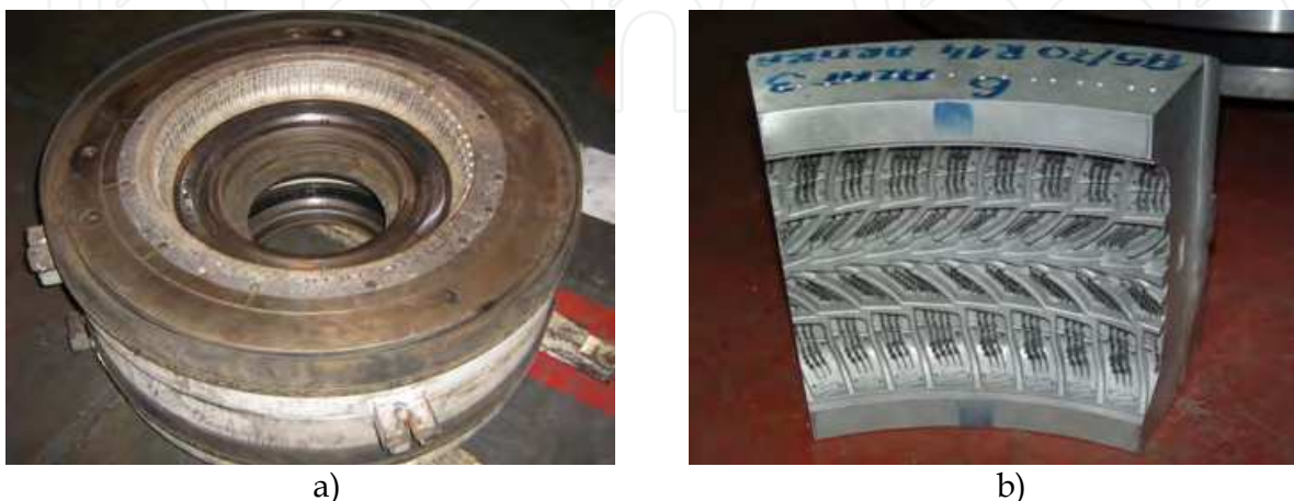
Fig. 5. a) Monoblock tyre vulcanization mould system b) 1/8 of tread ring segment.
