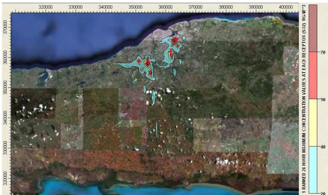
Fig. 9. Isolines of the maximum hourly concentration of \text{SO}_2 . (Source: Base Map Google Earth)
