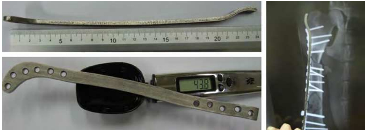
Fig. 23. Left: images showing size and weight of the customized plate. Right: post-surgery X-rays image of the plate (Courtesy of CIMA and FAUNA).
