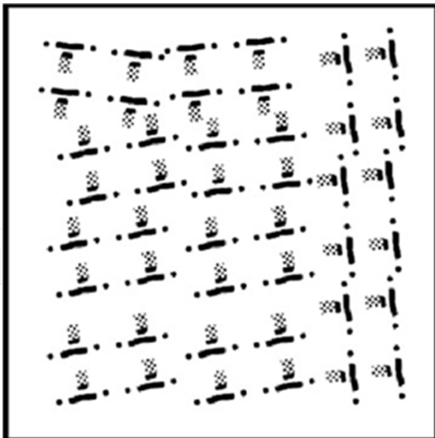
Fig. 11. One digital layer as represented in EBM Control software (black part is fused and white left unfused).
