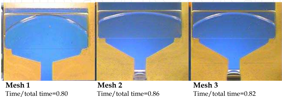
Fig. 6. Comparison of the effect of distributor geometry on the time it takes to reach the wall farthest from the injection port for vertical mould orientation.
