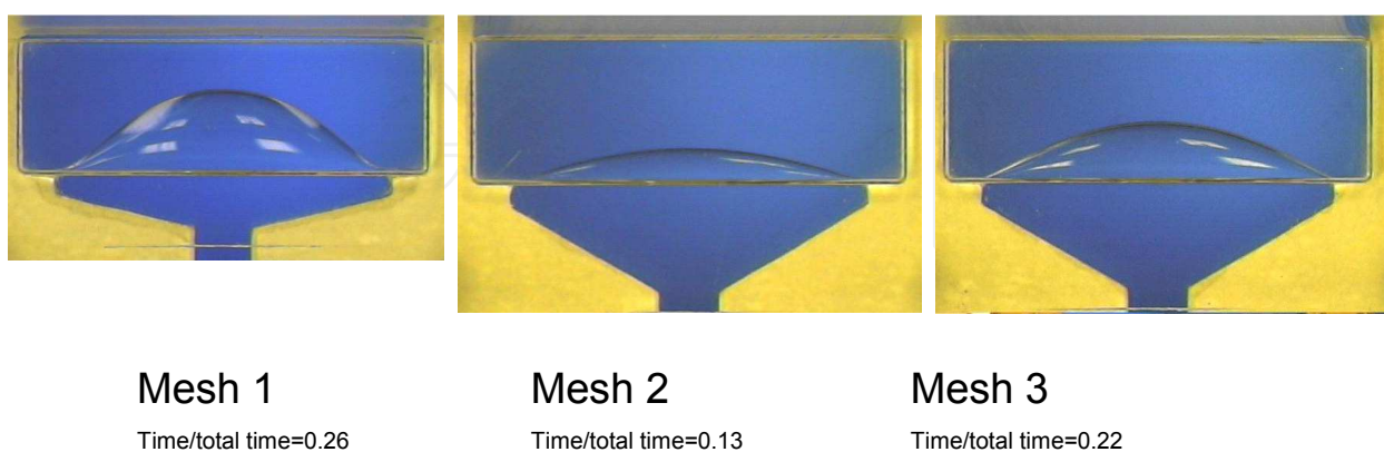
Fig. 9. Comparison of the effect of distributor geometry on the shape of the fluid front entering the mould in a horizontal orientation. The flow direction and gravity are perpendicular, with gravity acting in the thinnest cavity direction.
