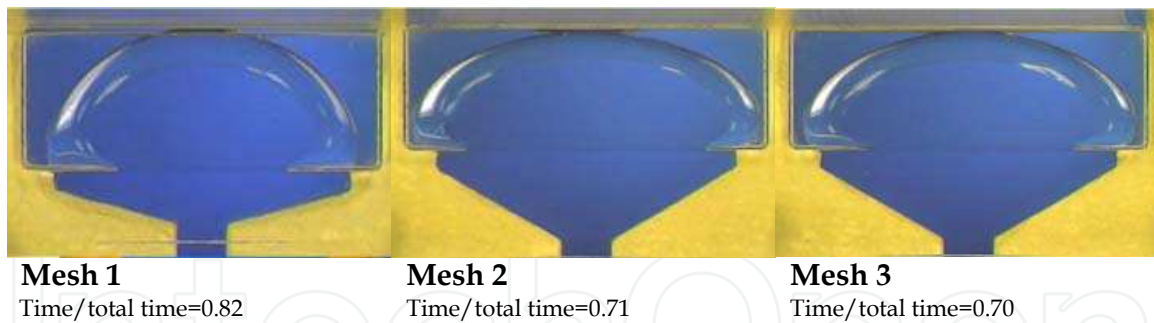
Fig. 10. Comparison of the effect of distributor geometry on the time it takes to reach the wall farthest from the injection port in a horizontal orientation.
