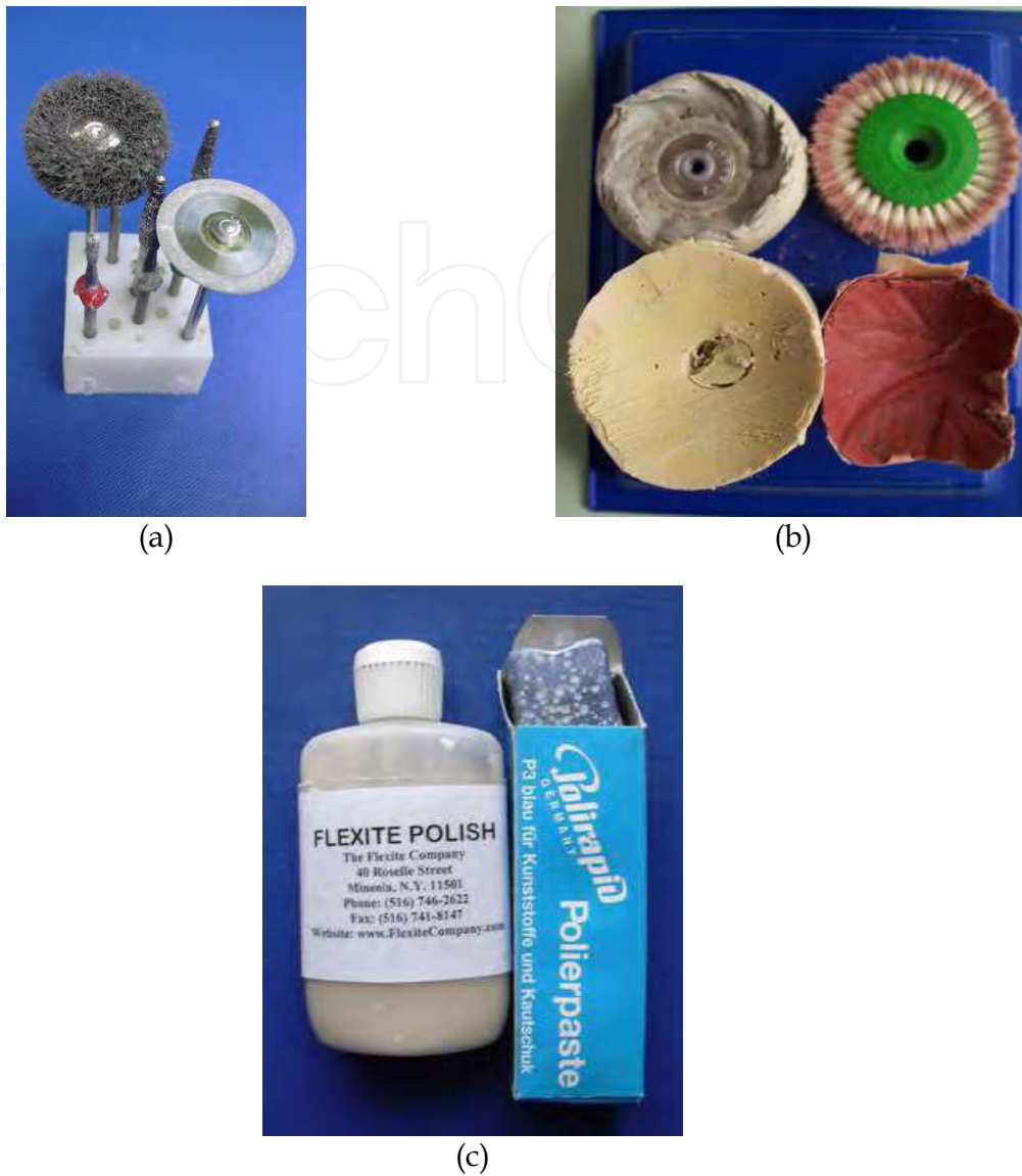
Fig. 13. (a) Tools used for processing the acetal framework, (b) Tools used for finishing and polishing the acetal framework, (c) Special polishing paste
