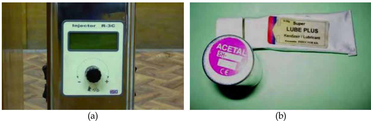
Fig. 10. (a) R-3C injector (Flexite), (b) The flask with grains of thermoplastic material and the lubricant used
