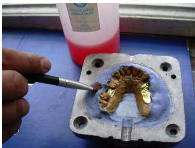
Fig. 9. Insulation of the investment
