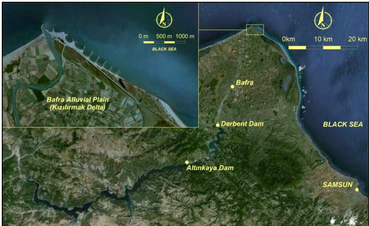
Fig. 3. Baфра alluvial plain and plan view of the existing shore protection system at the Kızılırmak River mouth (Google Earth, 2011)
