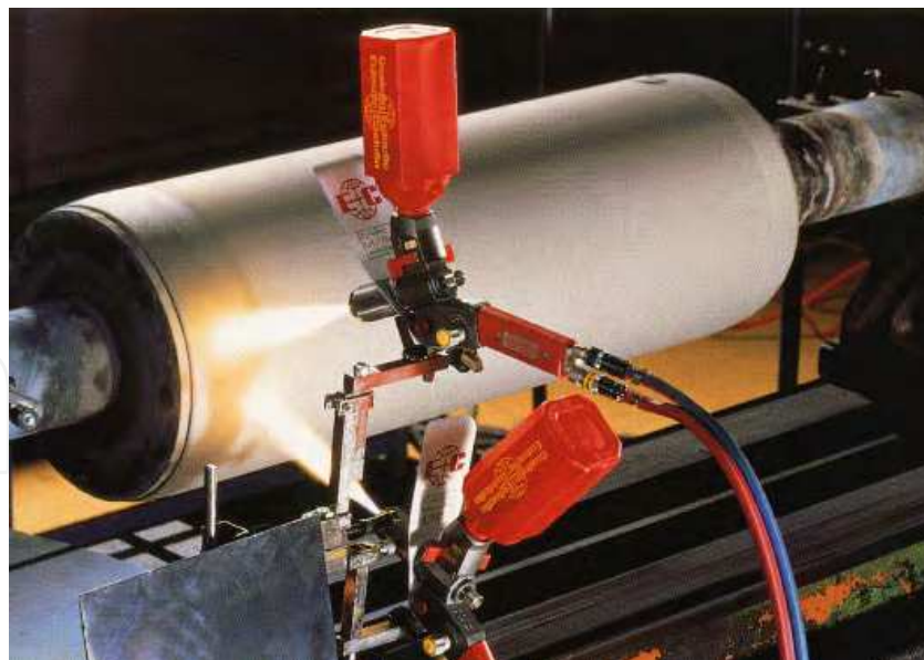
Fig. 7. Flame-coating of a cylinder used in food industry: 3-mm thick polyamide coating Ducos (2006) .
