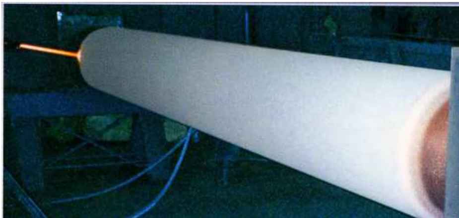
Fig. 8. Paper machine roll coated by NiCrBSi (self fluxing alloy) Vuoristo and Nylén, (2007) .
