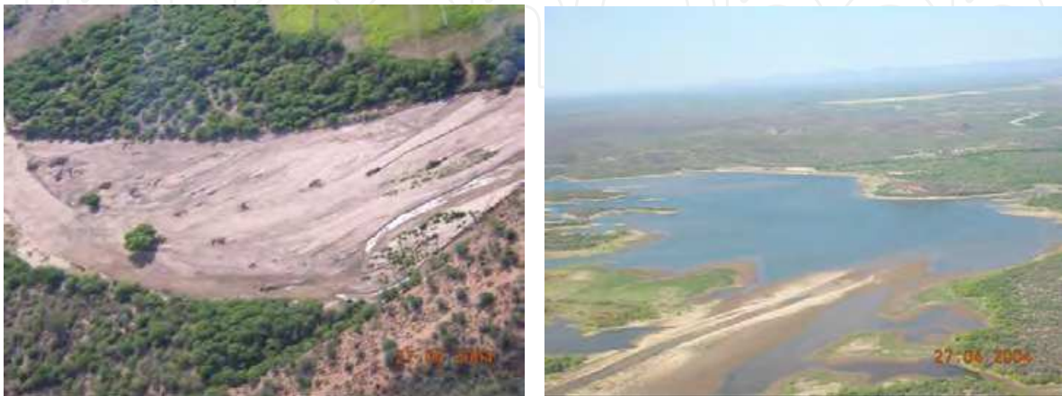
Fig. 10. Evidence of silting up in the Matapé River bed: 10a (left) a general widening and enhancement of river bed is observed; 10b (right) downstream, sedimentation is filling the dams reservoirs, threatening the irrigation downstream in the Coastal, semi-arid, plain.
