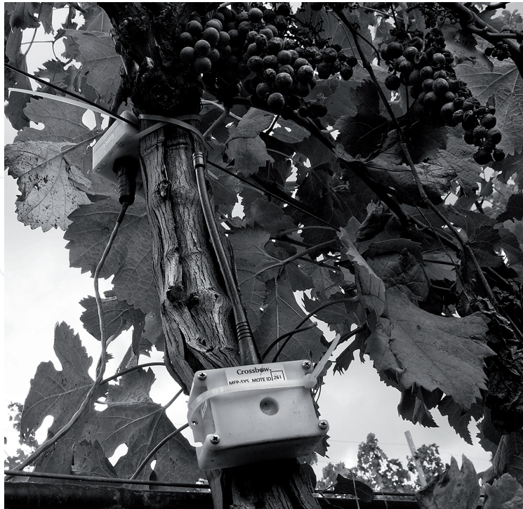
Fig. 2. WSN node attached to a vine in the Wisevine project.
