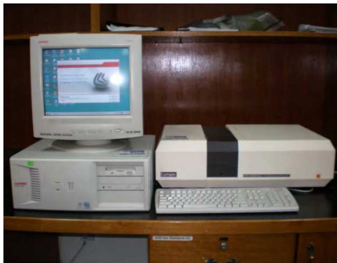
Fig. 3. The UV-visible spectrophotometer model Camspec M530. Faculty of Science, Department of Physics-UPM
