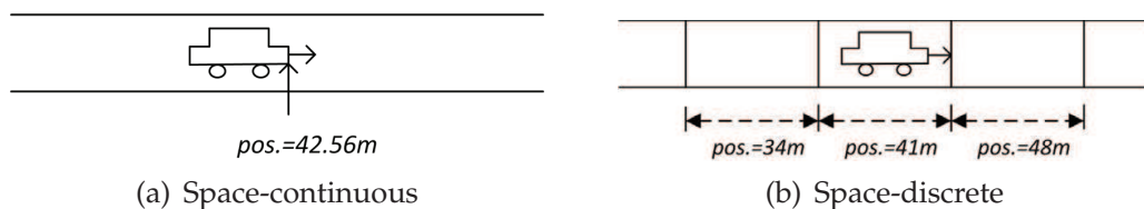
Fig. 5. The difference between space-continuous and space-discrete models.
