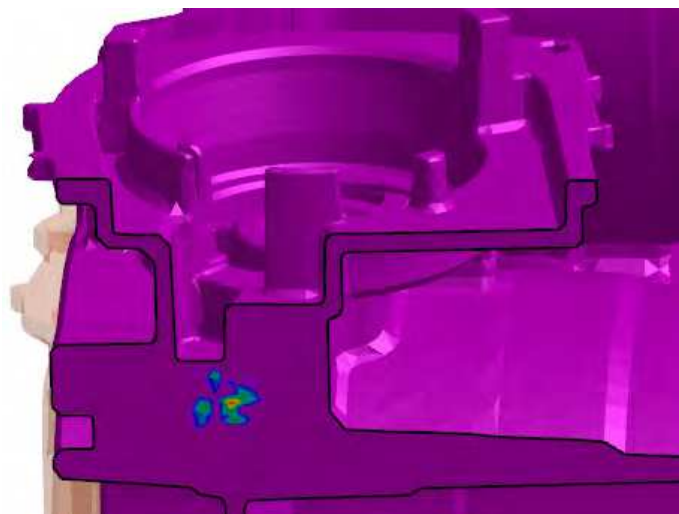
Fig. 13. (a, b) Shrinkage porosity simulation on left and right castings.
