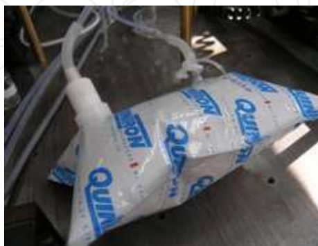
Fig. 20. Aluminum-coated plastic bag with sample gas.
