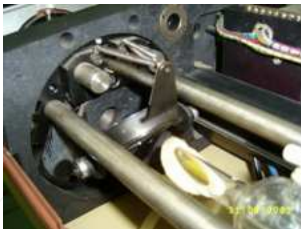
Fig. 6. Diffraction grating-drive mechanism.
