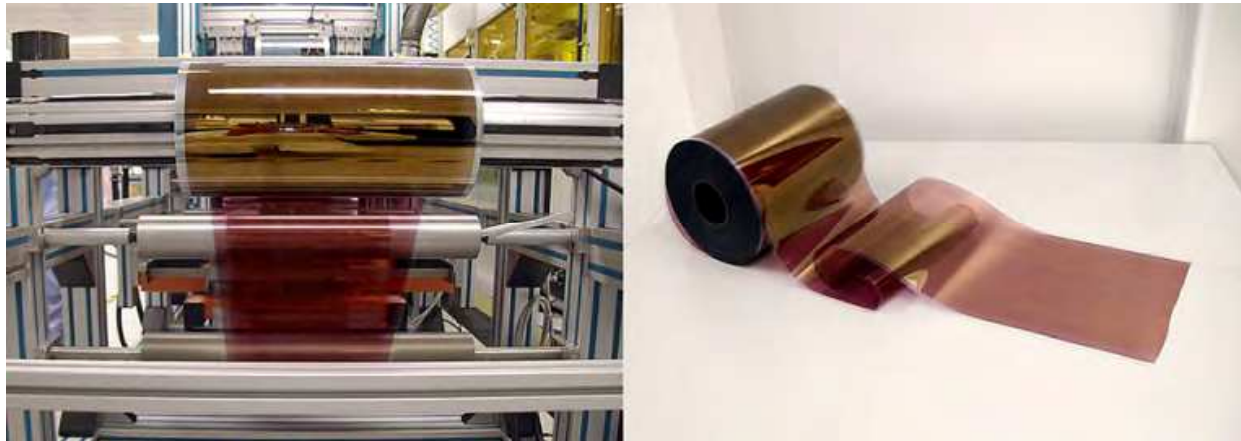
Fig. 2. Roll of the PET foil with slot die coated PEDOT and photoactive layers (reproduced with permission from (Galagan et al., 2011b), Copyright 2010, Elsevier B.V.).
