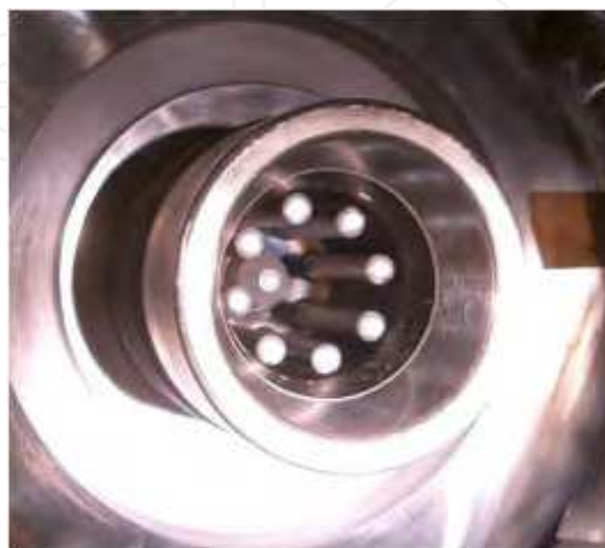
Fig. 8. Magnetoplasmadynamic(MPD) arcjet as solar wind simulator (SWS).
