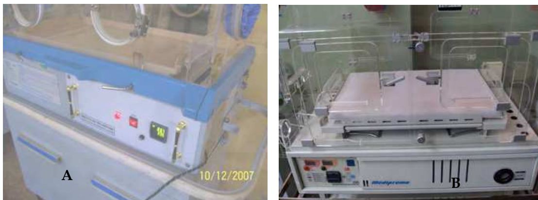
Fig. 4. Recycled incubators, originally carcasses of (A) Airshields model C200 (B) ISIS Mediprema system
