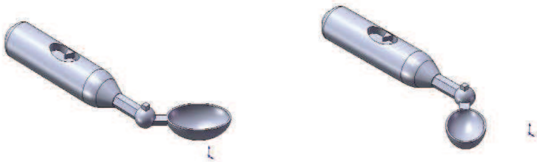
Fig. 4. New spoon could turn the shallow bowl to right and left side
