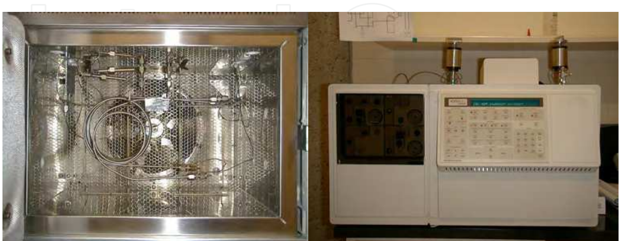
Fig. 5. Standard gas chromatograph and oven
