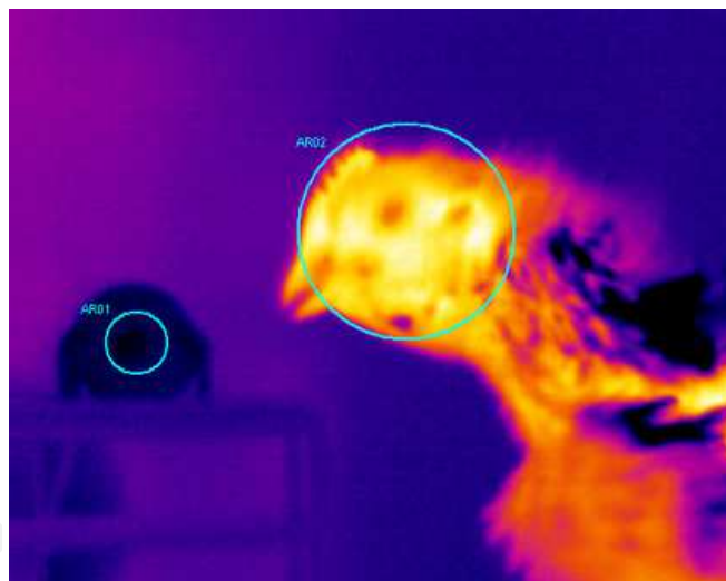
Fig. 6. Typical thermogram obtained in laboratory measurements. Two regions of interest were used for the analysis: one around the hole of the blackbody and the other around the hotter parts of the chicken's face. Camera software was used to read the minimal temperature of the blackbody cavity if it was colder than the surrounding, its maximal temperature if it was hotter than the surrounding, and its average temperature if the cavity was indistinguishable on the thermogram because the temperature differences were too small. For facial temperature measurement, the hottest temperature inside the ROI surrounding the face was recorded.
