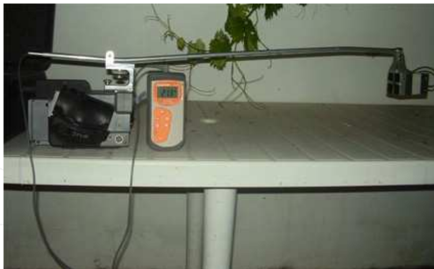
Fig. 4. Setting of field observations. The camera was attached in a permanent position at one end of a special "antenna", and the blackbody was situated at the other end, with the hole facing the camera. The distance between the lens and the blackbody was 80 cm. At the right-hand side of the picture can be seen the wire that connected a temperature probe that was inserted into the rear of the blackbody to the digital thermometer, which is displayed in front of the camera only for this photograph. During experimental measurements this thermometer was carried in a small bag, and the digital blackbody temperature was recorded manually for each thermogram.
