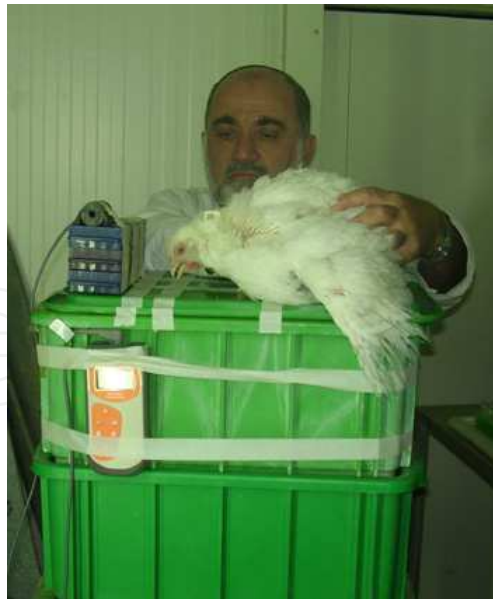
Fig. 5. Experimental procedure in the laboratory. The setting was identically arranged and located in each of the four climate-controlled rooms in which birds were exposed to various environmental conditions. The IR camera was permanently placed 80 cm from the blackbody.
