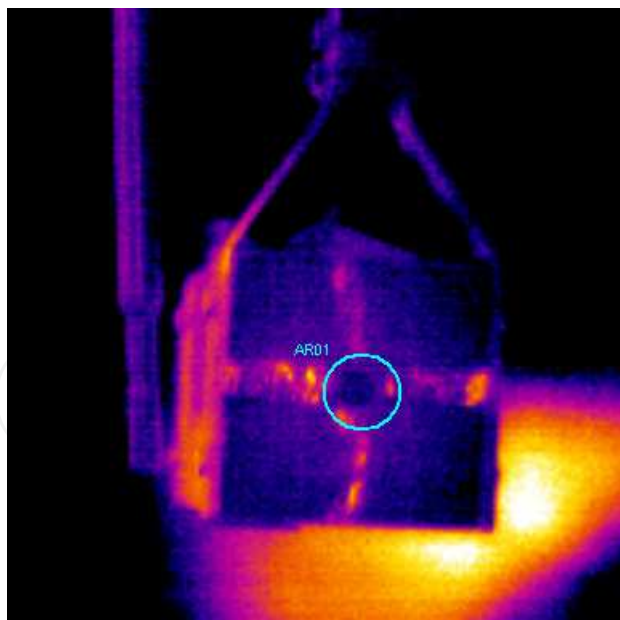
Fig. 2. Infrared thermography of the experimental setup for studying fluctuation of measurements. On the left side, the alcohol thermometer is visible. The blackbody is shown as a box in which the cylinder is confined. The hole of the blackbody cavity appears as a dark area, surrounded by the limits of the ROI (Region of Interest), as defined by the camera software. An electronic temperature probe which measured the actual temperature of the blackbody was inserted into the rear of the cylinder and is invisible to the camera.
