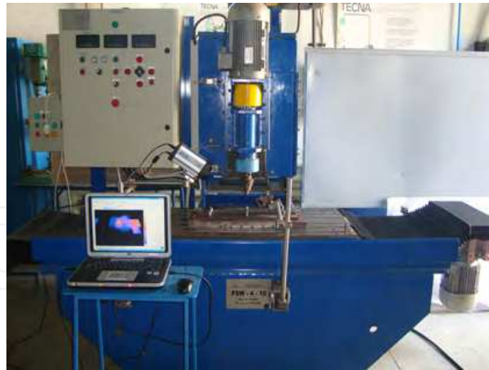
Fig. 22. FSW machine from ISIM Timișoara, Romania
