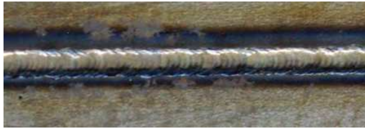
Fig. 20. Welded bead visual aspect for LASER-TIG variant
