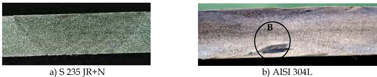
Fig. 31. Macroscopic aspect of welded joints
