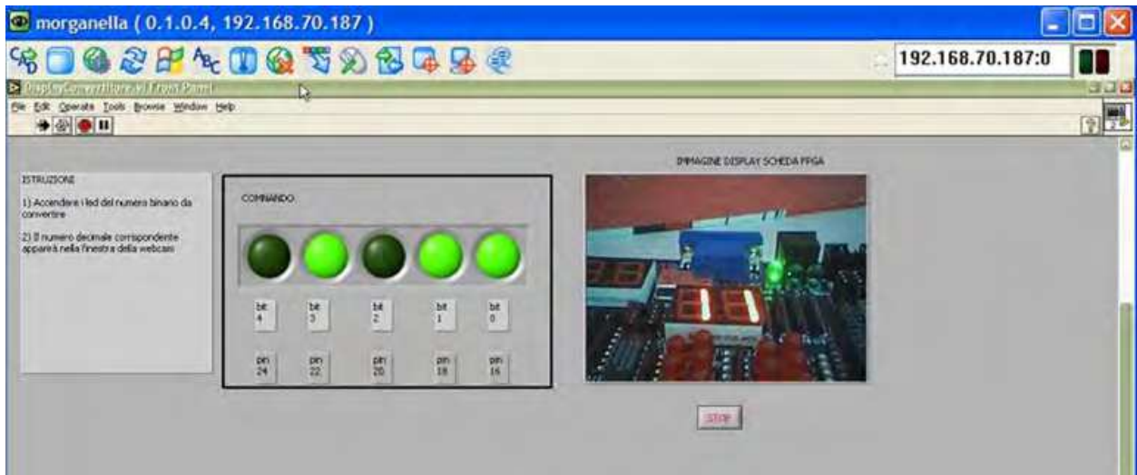
Fig. 9. Graphic user interface (GUI) of a binary-to-decimal digit converter.
