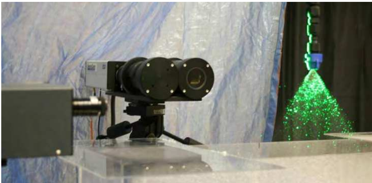
Fig. 6. Photograph taken during a PLIF imaging experiment utilizing a Dantec Dynamics FlowMap System Hub.
