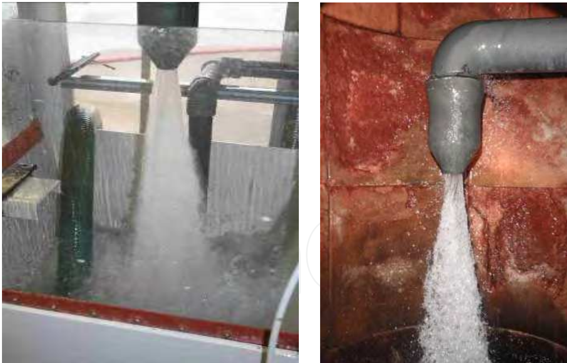
Fig. 2. Left, image of an axially-vented thermal quench nozzle in operation in the authors' test stand. The aim of this test was to quantify the spray angle and asymmetries of the plant nozzle. Several flow rates and nozzle designs were tested. Right, field test in plant.
