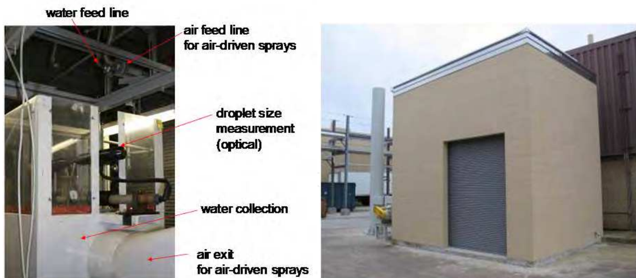
Fig. 1. Interior and exterior view of the nozzle test stand at The Dow Chemical Company, Freeport, Texas, USA.
