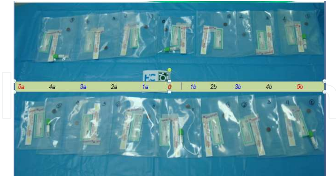
Fig. 6. Samples of packaging positioned from 0 to 5 for EtO penetration analysis.
