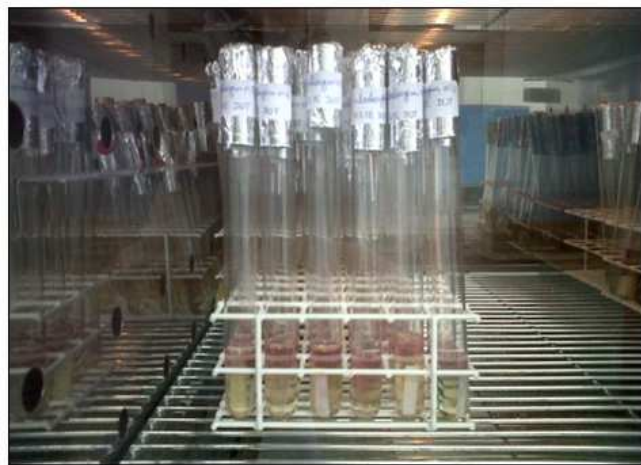
Fig. 7 and 8. Performance of the sterility test by direct incubation in samples submitted to ethylene oxide.
