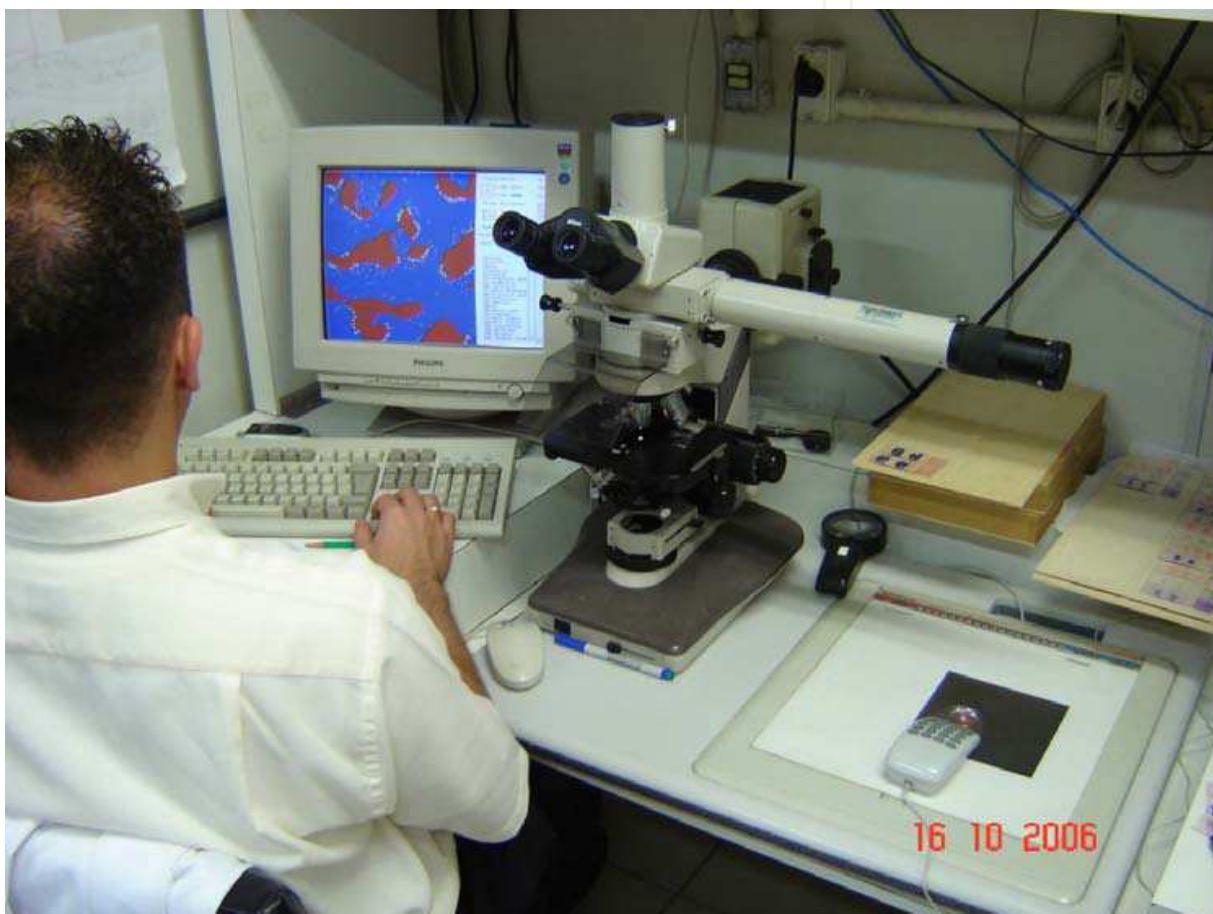
Illustration 14. Equipment used for histomorphometric analysis (microscope coupled to digitizing board and Osteomeasure® software)
