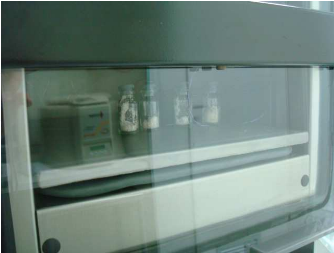
Illustration 11. Lyophilization chamber: Labconco® equipment from the Tissue Bank of Hospital das Clínicas - Universidade de São Paulo.
