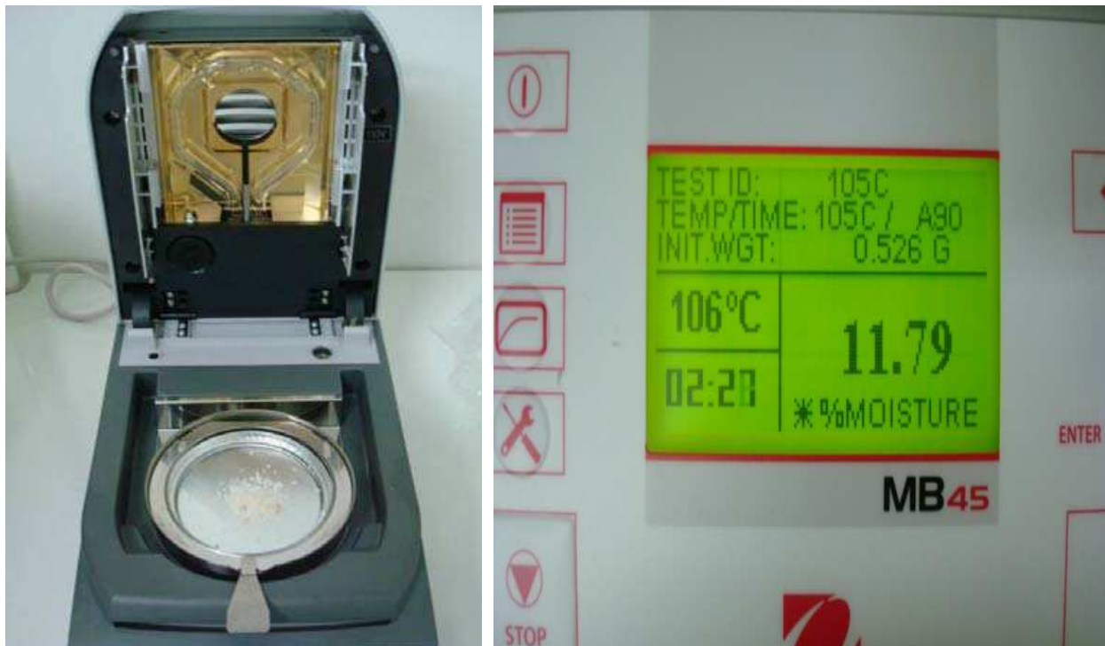
Illustrations 12,13. Residual Moisture Analyzer: Ohaus® equipment belonging to the Tissue Bank of Hospital das Clínicas - Universidade de São Paulo.
