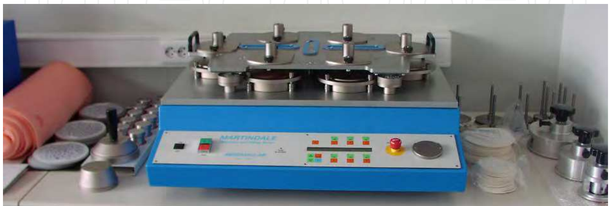
Fig. 1. Martindale abrasion testing apparatus
