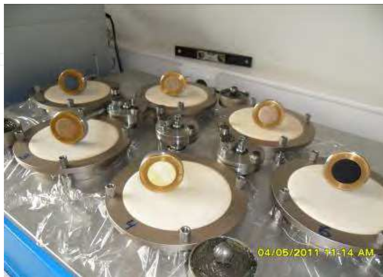
Fig. 6. Martindale abrasion tester prepared for wet abrasion
