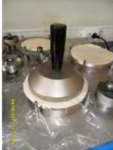
Fig. 5. Abrading table with a transparent film before clamping the ring
