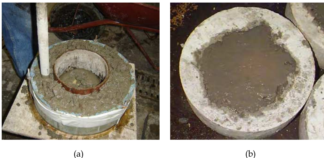
Fig. 3. Preparation of specimens for testing abrasion. (a) Release and compacting concrete reference. (b) System: substrate | repair material.
