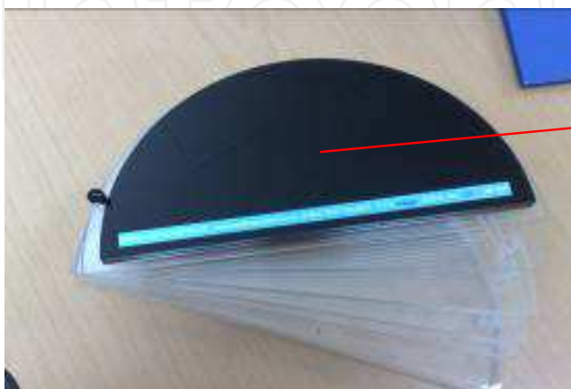
Image 1. ToRMAX-316 (Leeds Test Object).
