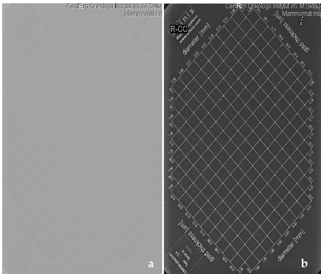
Fig. 3. Unprocessed image (a) and processed image (b) of CDMAM phantom for mammography unit 10 (unit 10 is the same as in Table 3).
